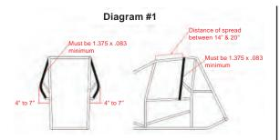
(b) Existing chassis with a left side support bar installed (formerly called safety bar) that do not meet the option one specification above, must add a gusset that attaches to the top rail 14" to 20" from the rear of the front up right and angle to the support bar. The existing support bar tubing must meet the minimum as described above (1.375 X .083 ASTM4130 normalized steel or equivalent material). See Diagram #2
