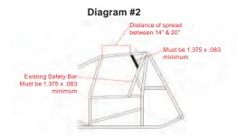
(c) A support bar must be added to the top rail at a point 14" to 20" from the rear of the front upright and to the rear upright near a point of the rear brace / shock mount bar but no higher than 7" above the hip rail. This bar must have a slight curve near the rear upright to accommodate elbow room and ease of fitment. See diagram #3
