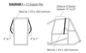
(2) Existing chassis with a left side support bar installed (formerly called a safety bar) that does not meet the option 1 specification above, may add a gusset that attaches to the top rail 14" to 20" from the rear of the front upright and angle to the support bar. The existing support bar tubing must meet the minimum as described above (1.375" x 0.083" Chrome Moly). See diagram 2
