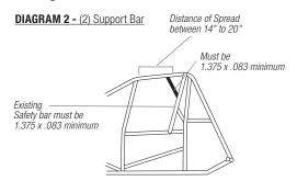
(3) A support bar may be added to the top rail at a point 14" to 20" from the rear of the front upright and to the rear upright near a point of the rear brace/shock mount bar but no higher than 7" above the hip rail. This bar may have a slight curve near the rear upright to accommodate elbow room and ease of fit. See diagram 3.
